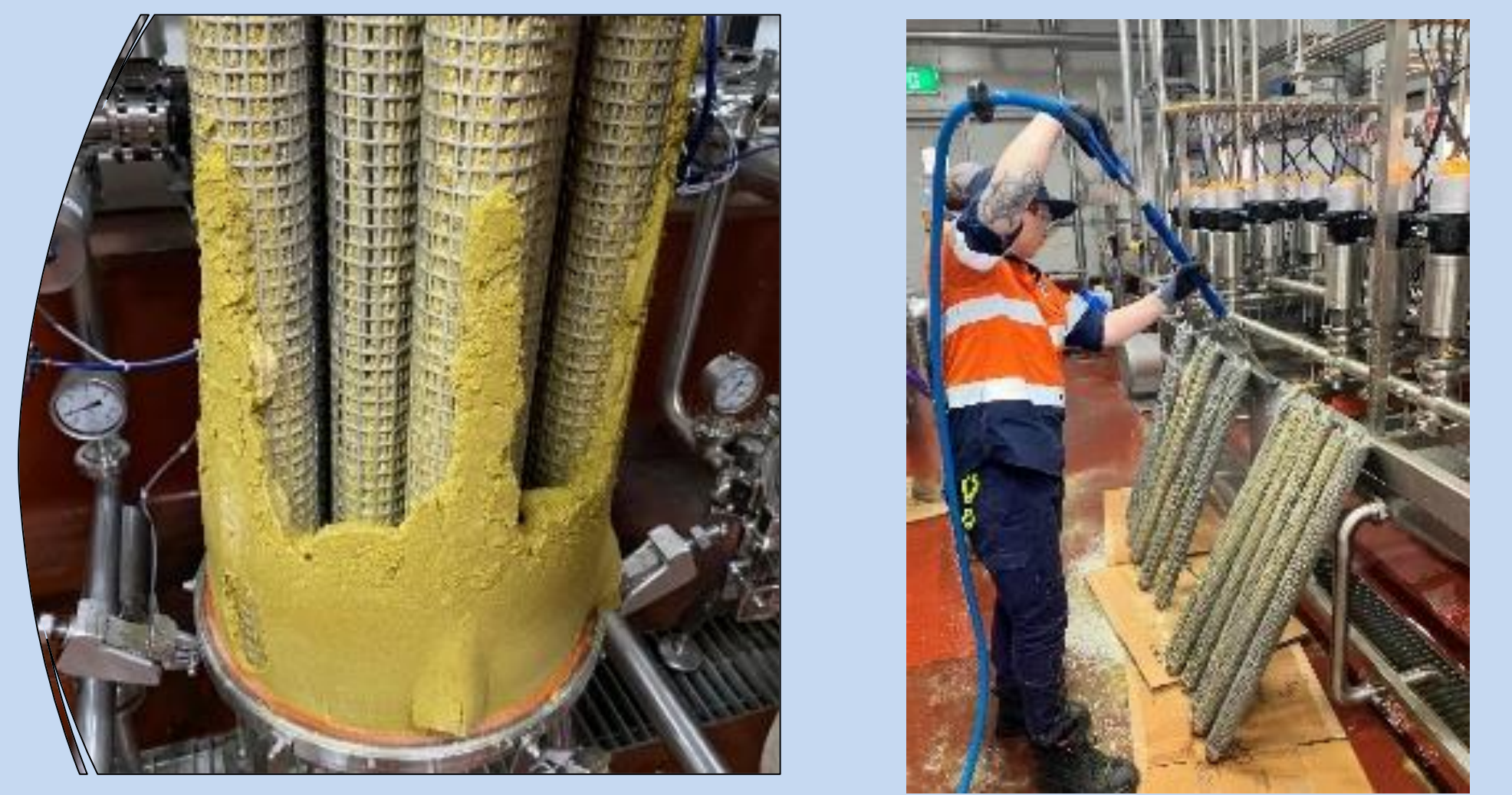
Figure 1 Blocked 100µm Strainers en-route to glass and keg line and manual cleaning process required if they block up.
